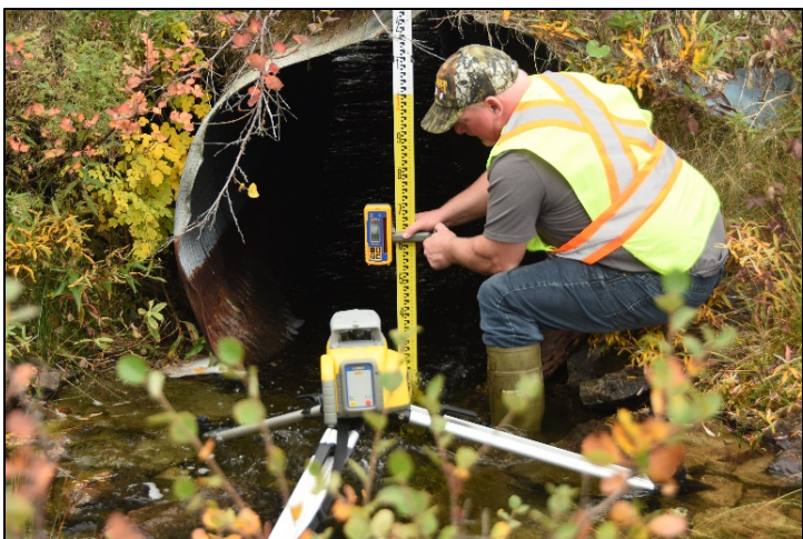
Jake Sinnicks using the self-leveling laser kit to measure inlet elevation at culverts on the Northern Peninsula.
